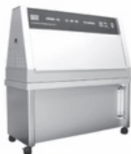
QUV Accelerated Weathering Tester - Uses Fluorescent UV lamps to reproduce the damaging effects of sunlight.
