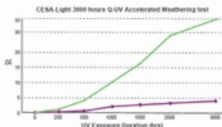
After 3000 hours Q UV, ΔE of VULCAN Polycarbonate sheet is at 3 to 4.
