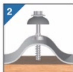
2 A perfectly round nominal 11mm diameter hole is created by the Thermal Expansion Hole Cutter during the process.
