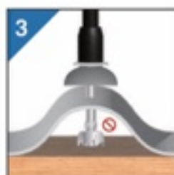
3 The Expansion Hole Cutter works in combination with the Depth Stop Knurls, and prevents overdriving of the screw after touching the purlin.
