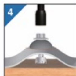
4 A large Domed Weatherseal EPDM washer with two concentric sealing rims on the washer underside completes the package.
